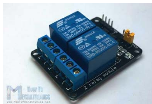
Fig. 6. HL-52S 2 channel relay module showing output connector
