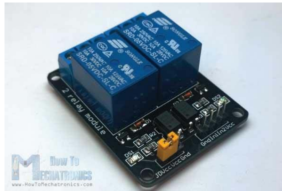
Fig. 7. HL-52S 2 channel relay module showing input pins
